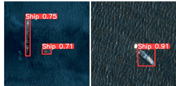
Figure 4: SR-YOLOv5 vessel detection
